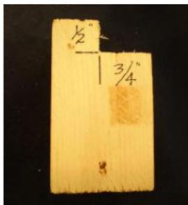
Another useful tool is a 2 x 2 block of wood with a notch in one end. It backs up the tin while center punching the holes. Clamp in a vice and it will make cleanly center punching the holes much easier.
