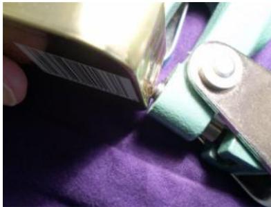
Screw the 1/4" die in the bottom jaw, and insert the 1/4" punch in the top (movable) jaw. If you have the metric version use the 6mm set. You will have to gently use a round file or tapered reamer to slightly enlarge the holes for the jack's threads. Slide the end of the tin into the jaw taking care not to scratch it with the point on the punch.
