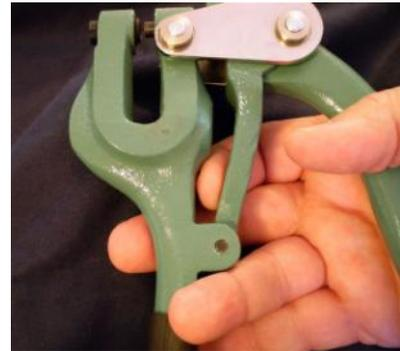
***The key to accurate punching is to bring the tin to the punch and nestle the dimple on the point of the punch before squeezing.***
