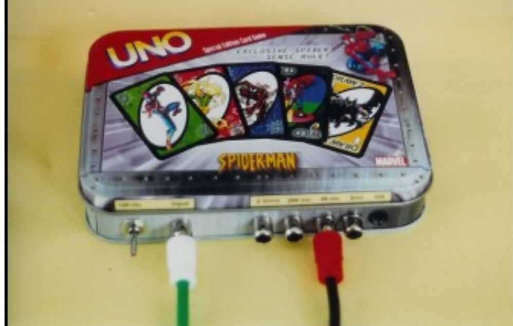
Notice all the phono jacks. The signal injector and the signal tracer have different colored heat shrink tubing.
