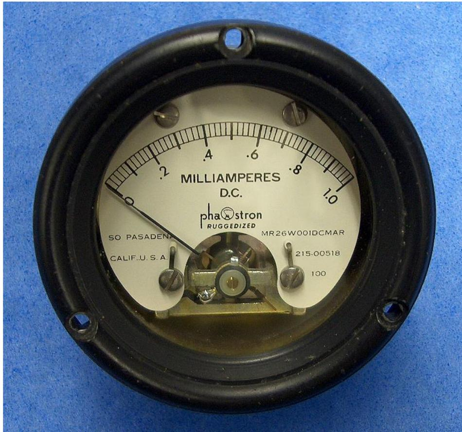
Well, the meter range is about right - the reading of 100 ma that I need to see is easily readable, and the full scale reading of 1 ampere would make the meter usable for testing with higher powered gear. But, since the DC meter cannot read RF, what to do?
